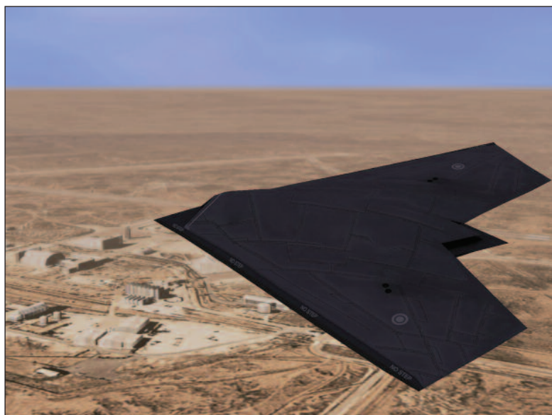
The BAE Systems Taranis, a semi-autonomous unmanned warplane utilising stealth technology, is able to attack both aerial and ground targets while on intercontinental missions.
